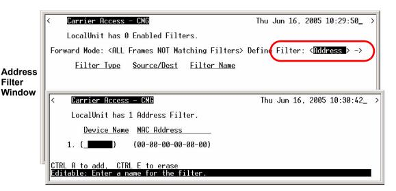
Use this window to define filters that are based on the Ethernet MAC Address of a specific device. When enabled, these filters provide security by restricting LAN/WAN access based on a device's MAC Address. Address filters are based on either source. destination or both source and destination MAC Addresses.
